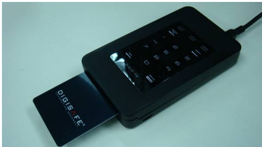
Insert the smart card into the smart card slot with the contacts facing down and the word “DigiSAFE” on the card facing up
